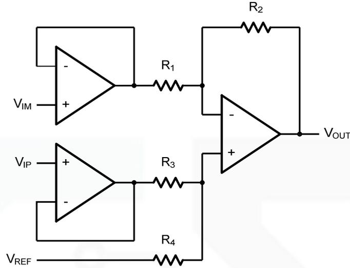
Figure 6. Instrument Amplifier
